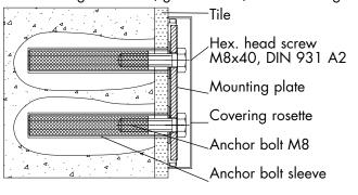
6 hex. head screws6 anchor bolts6 anchor bolt sleeves(Fischer assembling mortar360S provided by the customer)
